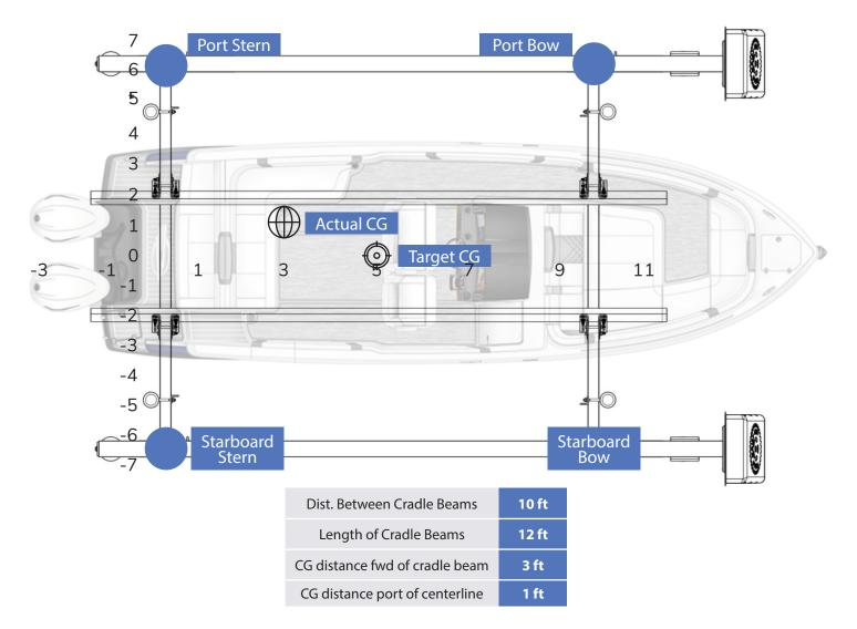
With the CG at this location and for this "wet" boat weight, the picture below shows the tension in each vertical wire rope.
