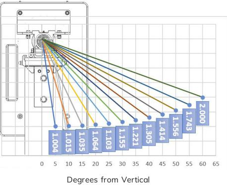
The cable may be 5° from vertical when the lift is fully lowered but depending on the geometry of the installation, the cables may be at 35° from vertical when the lift is fully raised. The tension will increase from 1.004 times the straight-line vertical tension to 1.221 times (22.1%).
