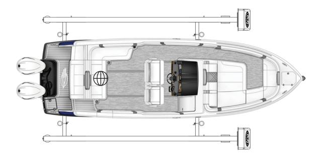
Additionally, the tension in the cable will increase if the CG of the boat is not centered between the cable lift points and will be highest on the cable that is closest to the CG location.
