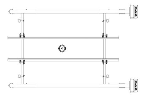
The ideal location of the CG is centered between the cradle beams and side to side, the CG of typical power boats tends to be over the after 1/3 as shown which means the tension is greater toward the after end.
